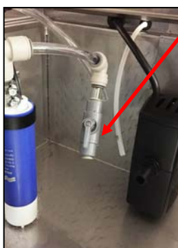
Fig. 3 Priming valve in OPEN position
