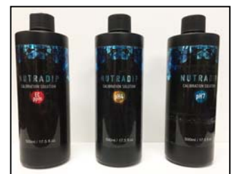
TDS 1000 EC ppm solution: To calibrate total dissolved solids probe
