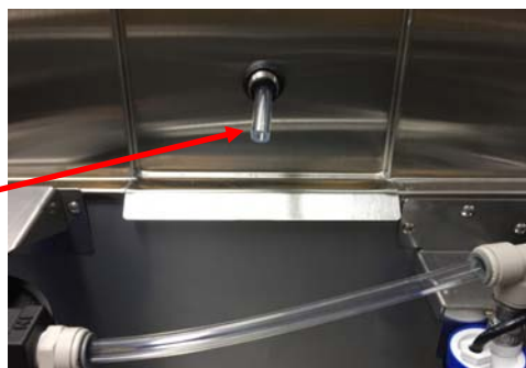
Fig. 5 Zone irrigation nozzle
