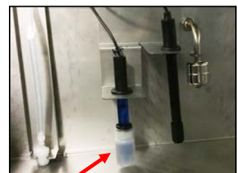
Fig. 2 Blue PH sensor (shown with cap on)
