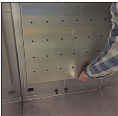
Fig 2. Remove rear duct
