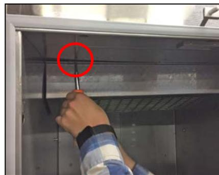
Fig 4. Evaporator cover screws in front (3)
