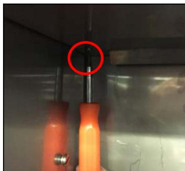
Fig 3. Evaporator cover screws in rear corners (2)
