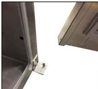
Fig 4. Lift door/bottom pin
